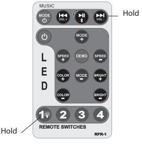
**Step 2.** Press and hold the and buttons. After 5 seconds you will see that the red led on the remote will start to flash slowly. Once the led is flashing release the buttons
